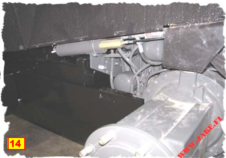
Tankin takakiinnitys. Rear end fastening of the tank.
